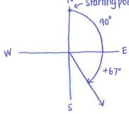
(2) The other system starts with a north or south line and uses an acute angle to show direction. The angle given is **measured from the second direction to the first**.
