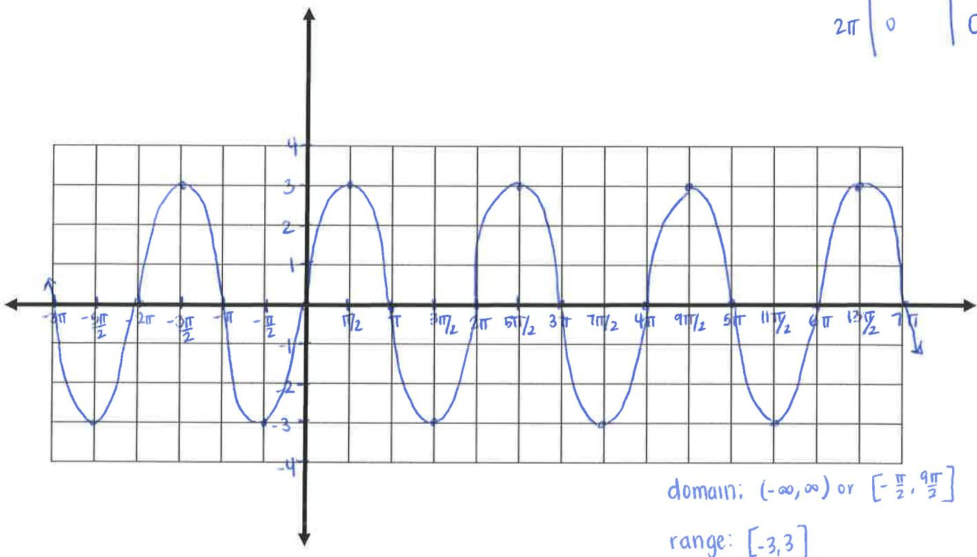
The amplitude of a function is half the distance between the maximum and minimum values of the function.
