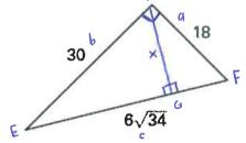
Step 2 Draw in the altitude to the hypotenuse. Identify the similar triangles and sketch them so that the corresponding angles and sides have the same orientation.
