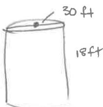
$$\begin{aligned} SA &= 2\pi r^2 + 2\pi rh \\ &= 2(3.14)(15^2) + 2(3.14)(15)(18) \\ &= 1413 + 1695.6 \\ &= 3108.6 \text{ ft}^2 \end{aligned}$$
